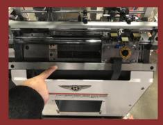
The head of the machine is connected to the pedestal without the use of pull rod and motor, which greatly lightens the load of the machine
