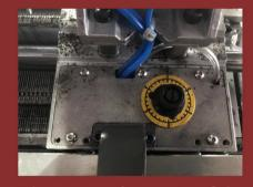
The connecting parts of the head and the pedestal are adjusted by four bearings so that the machine can be easily rotated back and forth, and at the same time, the adjustment clearance with the needle plate is more reliable.
