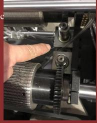
The worm gear and worm gear adopt the function of individual adjustment, so that the machine can adjust conveniently and quickly and accurately control the precision in the debugging process.
