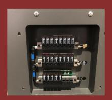
Using High Precision High Frequency Solenoid Valve to Control Pneumatic device Fork and scissors drives are driven by synchronous wheels and stepping motors, and the position of the fork and scissors is more accurate
